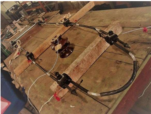
Ageing test of Insulation Piercing Connectors
