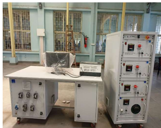
CB Analyzer cum Mechanical Endurance Test set
