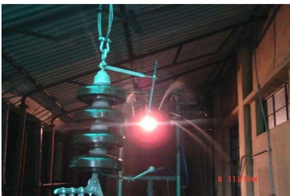
High Voltage (Wet) Test of Porcelain Insulator
