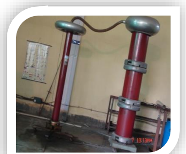
HV Power Frequency Test Set
